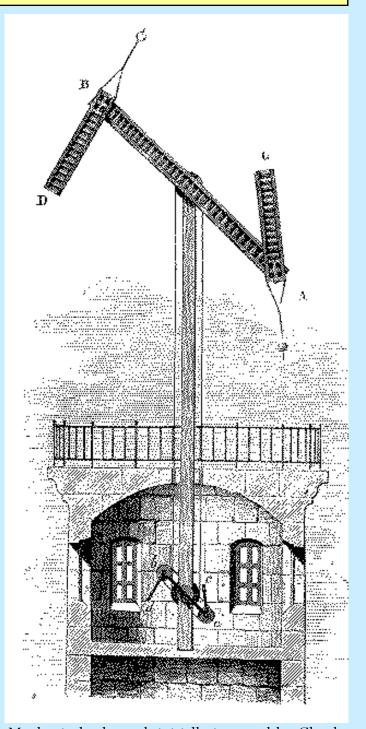
Mechanical telegraph initially invented by Claude Chappe and popularized in Dumas' novel, *Le Comte de Monte Cristo*. The *stationnaire*, by working the inside apparatus, moved the arms and cross-support to form figures representing coded signs.
